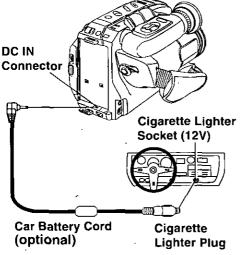
Connect PV-C16 Car Battery Cord (optional) to Camcorder DC IN.
